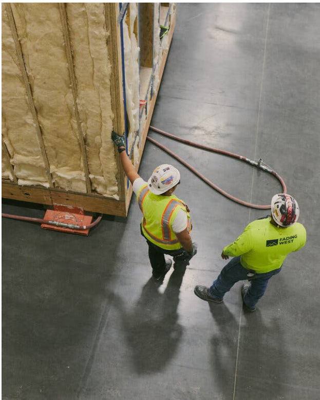
Wooden platforms the size of train cars move the housing units from one station to the next.
